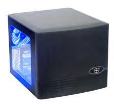
With up to ten 3.5" drives, or as many as twenty-two 2.5" drives *inside* the enclosure, this platform is an ultra-dense solution. Up to 60TB of disk, or over 40TB of enterprise high-performance SSD, are packed into a form factor that easily fits on or under a desk.
